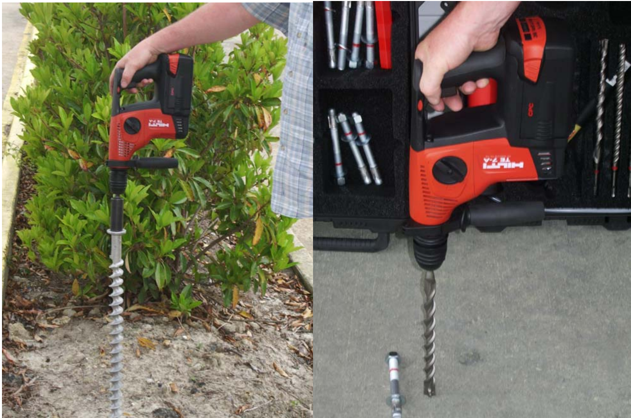
HILTI CORDLESS TE 7-A WITH AMERICAN EARCH ANCHOR (LEFT) HILTI CONCRETE DRILL BIT (RIGHT)
